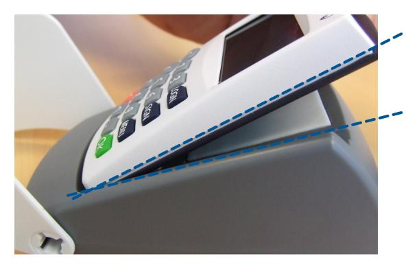
Place the DIGIPASS 870-875 in the smallest possible angle, without touching the double sided tape
