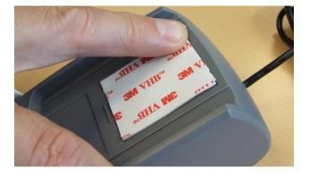
Firmly press the tape to have maximum adhesion
