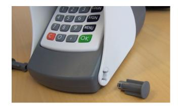
It is very important to place the plastic axes first time right. When wrongly inserted, the privacy shield will be permanently fixed and it is no longer possible to flip the privacy shield.
