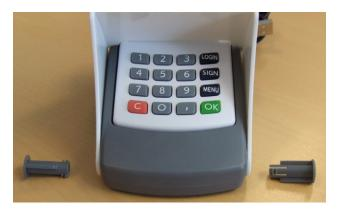
It is very important to place the plastic axes first time right. When wrongly inserted, the privacy shield will be permanently fixed and it is no longer possible to flip the privacy shield.
