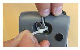
Hold the cable in the cavity while fastening the cable tie
