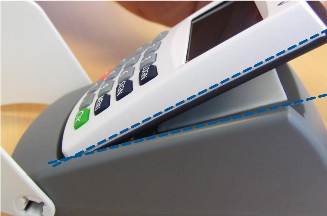
Place the DIGIPASS 870-875 in the smallest possible angle, without touching the double sided tape
