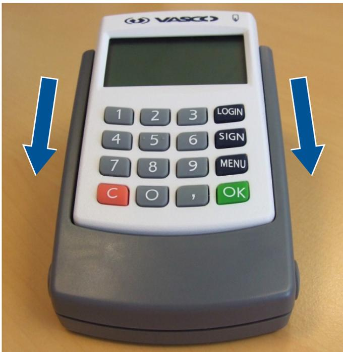
Slide DIGIPASS 870-875 in the cavity until a firm “click” from the connector is heard and felt.
