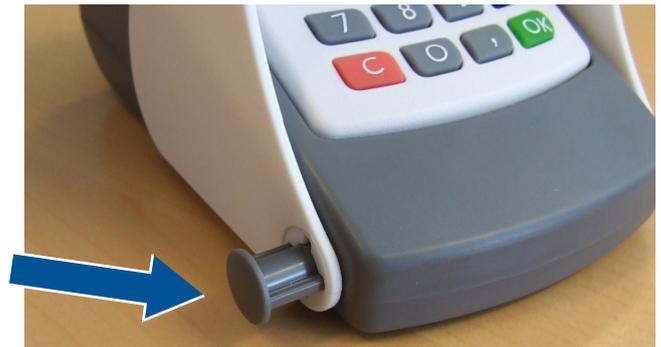
Make sure the ridges on the axis are in horizontal position!
