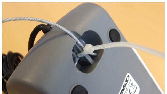
Hold the cable in the cavity
