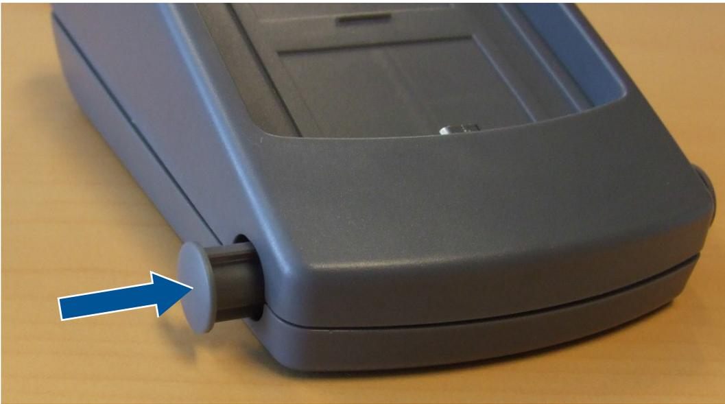
Make sure the ridges on the axis are in vertical position! This is done for both sides of the cradle.
