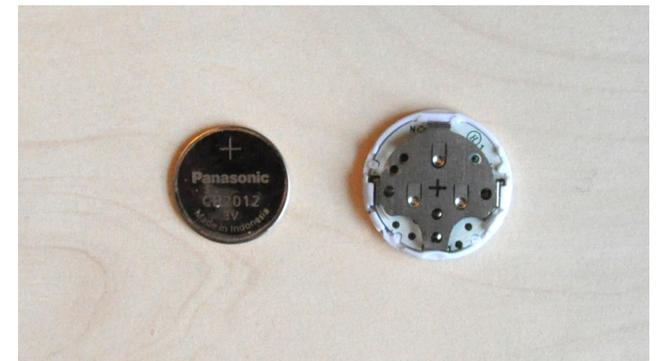
5. When re-attaching the two sides of the device, carefully align the (3) slots on the side and gently press to secure the two sides together.
